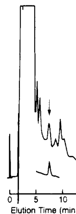
FIGURE 5: Analysis of the products formed from d-(CGCTTTAAAGCG) following successive treatments with Fe(II)·BLM A 2 and alkali. The arrow indicates the position of elution of a peak that comigrated with authentic dinucleotide 1 (inset) when analyzed by anion-exchange HPLC. Sample analysis was carried out on a 25-cm Du Pont Zorbax Sax anion-exchange column; elution was with 0.05 M ammonium phosphate buffer, pH 4.5, at a flow rate of 2 mL/min (monitored at 254 nm).
